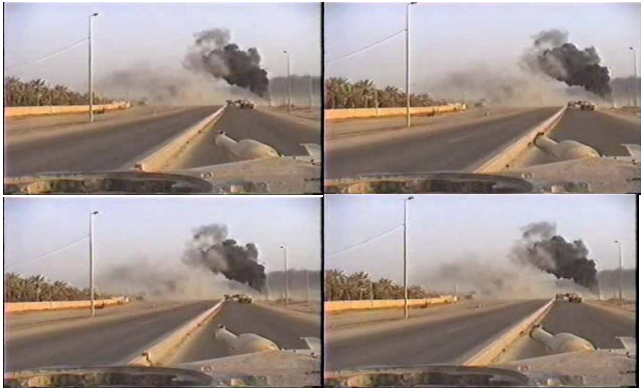
Figure 9: (Top Left) Source Video Stream, (Top Right) Quality at destination 1 hop away, (Bottom Left) Quality at destination 2 hops away, (Bottom Right) Quality at destination 3 hops away
